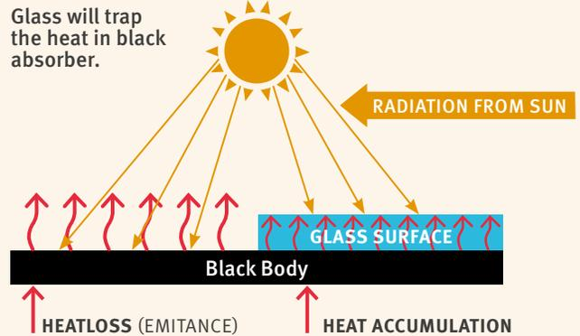
**CONCEPTUAL DIAGRAM OF SOLAR HOT AIR GENERATION**
