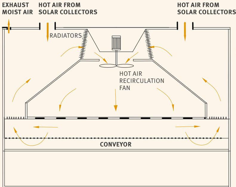
CROSS SECTION VIEW OF AN AUTOSPRAY DRIER WITH THE INTRODUCTION OF SOLAR HOT AIR.
